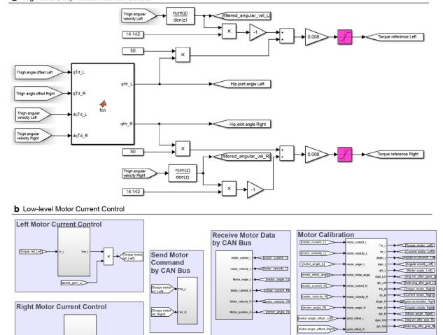
**Supplementary Fig. 2 | Exoskeleton control diagram. a,b**, The exoskeleton was electrically connected to a target PC computer with a Simulink Real-Time system (MathWorks, Natick, USA) running both a high-level neural network control (a) and a low-level motor control module (b).
